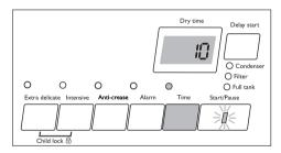
2. Press the *Time* button repeatedly until the desired programme duration is shown in the display, e.g. 20 for a programme of 20 minutes.
